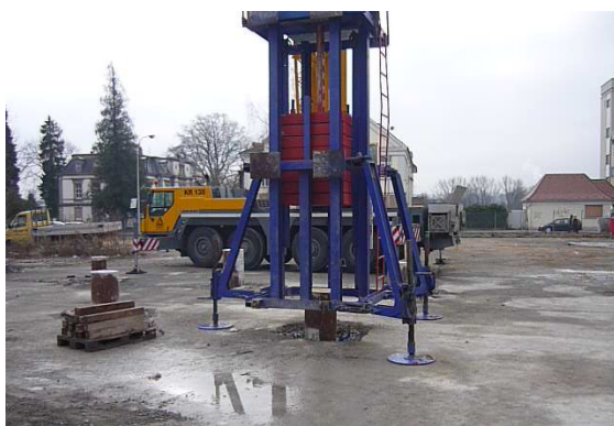
Figure 4. Free-falling weight for dynamic loading tests
